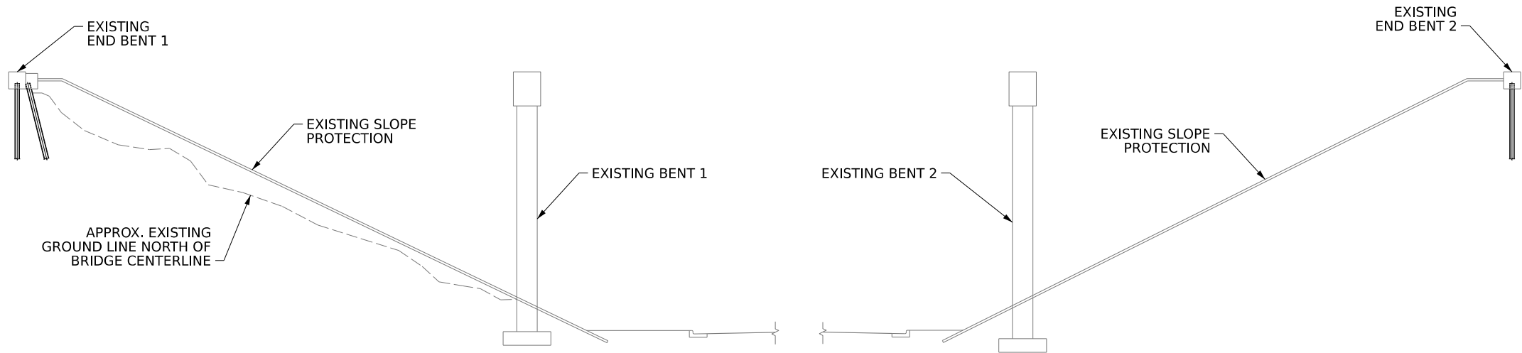
EXISTING SECTION ALONG CL (NBL)
